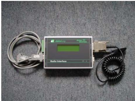
The **deprotect** system is designed to work with the **Central Station Radio Interface WK1204** and the user-friendly on-line software that runs on Windows 98, NT, 2000 or XP. The WK1204 radio interface has been specially developed to cipher high security data encrypted data transmission between the **Central Station** location and **deprotect**. The software monitors time, location and
